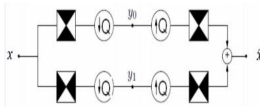
Figure (6). Two-dimensional spectrum partitioning using quincunx filter banks with fan filters. The black regions represent the ideal frequency supports of each filter.  $Q$  is a quincunx sampling matrix.
