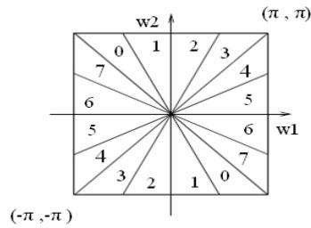
Figure (5) Directional filter bank. Frequency partitioning where  $l = 3$  and there are  $2^3 = 8$  real wedge-shaped frequency bands. Sub-bands 0–3 correspond to the *mostly horizontal* directions, while sub-bands 4–7 correspond to the *mostly vertical* directions.
