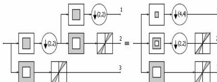
Figure (8). Block diagram of the contourlet transform with two levels of multiscale decomposition. Gray regions represent the ideal pass band support of the component filters. Left: The iterated form. Right: The equivalent parallel form.
