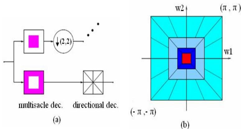
Figure (1) the original contourlet transform. (a) Block diagram. (b) Resulting frequency division
