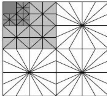
Figure (3) plot of the WBCT using 3 wavelet levels. The directional decomposition is overlaid the wavelet sub bands.
