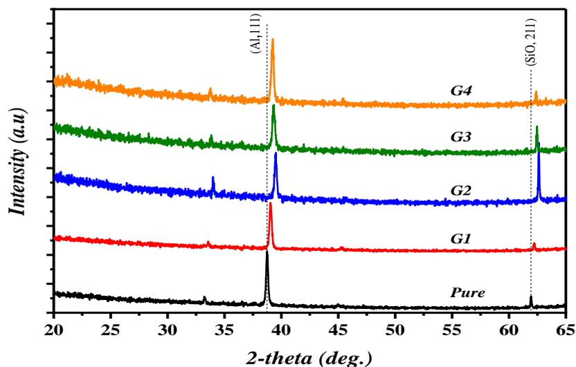
**Fig. 1: XRD patterns of the Pure MOS and Gamma irradiation MOS structure.**
