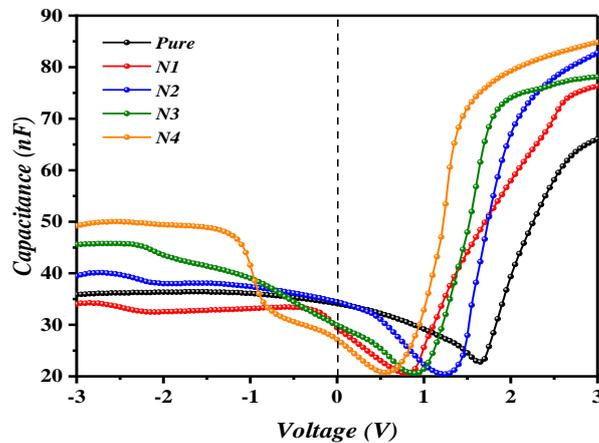
Fig. 7: C-V characteristics for pure MOS and neutrons irradiated MOS structures.
