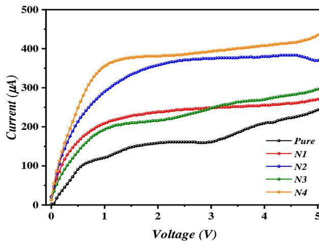
**Fig. 5: I-V characteristics for pure MOS and neutrons irradiated MOS structures.**
