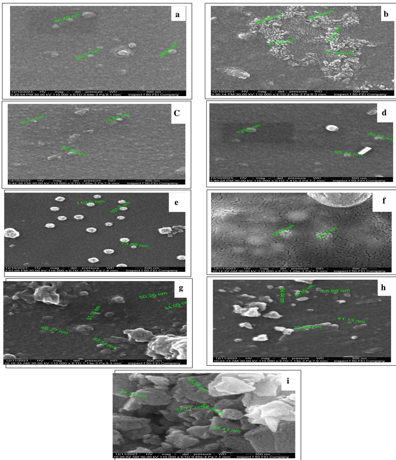
**Fig. 3:** The obtained FE-SEM images for (a) Pure/pristine, (b) 10 days gamma irradiation, (c) 20 days gamma irradiation, (d) 30 days gamma irradiation, (e) 40 days gamma irradiation, (f) 5 days neutrons irradiate, (g) 7 days neutrons irradiate, (h) 9 days neutrons irradiate and (i) 12 days neutrons irradiate.
