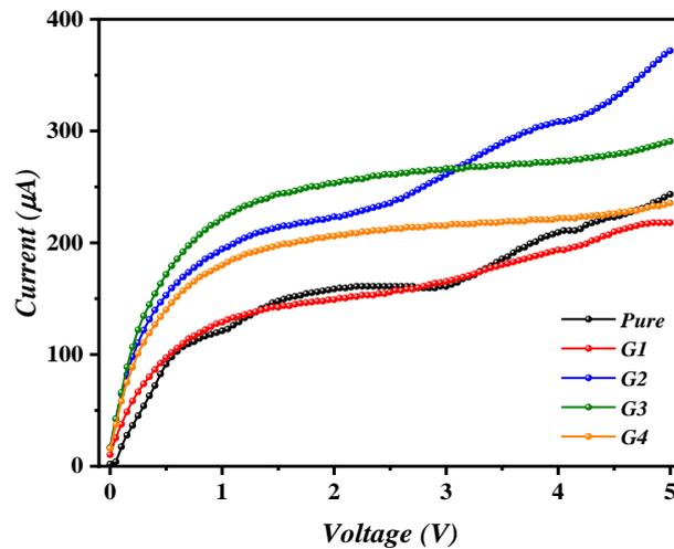
**Fig. 4: I-V characteristics for Pure MOS and gamma irradiated MOS structures.**
