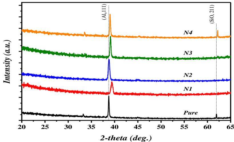
**Fig. 2: XRD patterns of the Pure MOS and neutrons irradiation MOS structure.**
