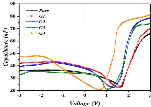
Fig. 6: C-V characteristics for pure MOS and gamma irradiated MOS structures.
