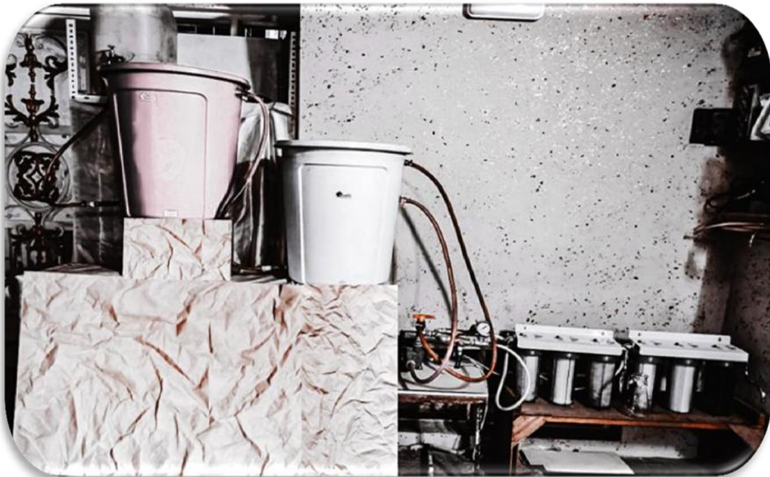
Fig. 1: A Lab scale wastewater treatment plant using modified Nanofilter
