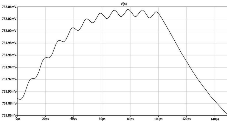
**Fig. 9: Simulated time domain transient analysis of the output voltage signal. Output voltage in (mV) and time domain in (ps).**
