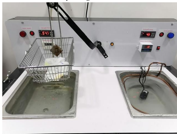
Figure (3): Alternating thermal-cycling machine/ Readymade, Iraq
