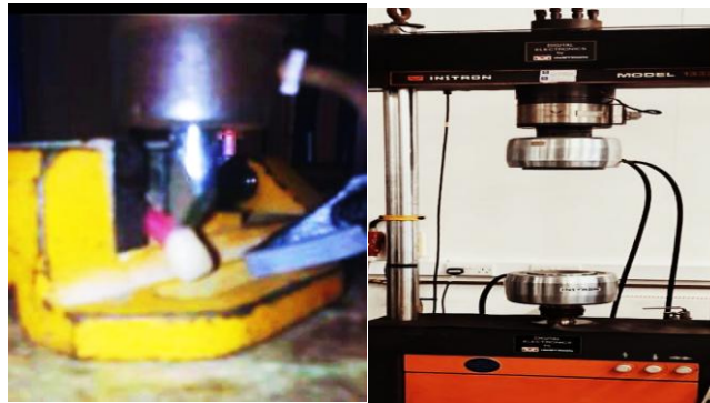
Figure (4): Universal testing machine (Instron Model 1332 Servo Hydraulic Fatigue Test System 100kN Load Cell 2513-502)
