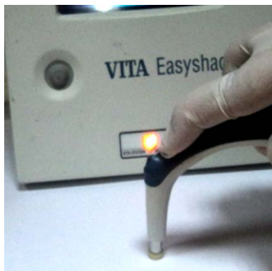
Figure (2): Method of color measurement for composite resin sample
