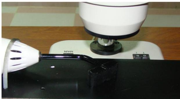
Figure (1): Metal base (black) holding the composite mold and the light cure unit under the stereo microscope.
