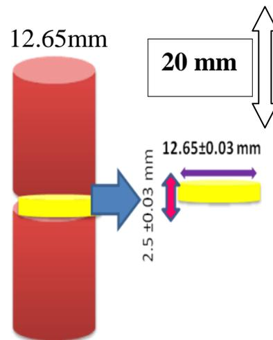
Figure (2): Pair of acrylic cylinders+ Rounded metal spacer
