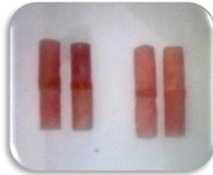
Figure (3) : Two Pairs of acrylic cylinders with Vertex and Molloplast-B lining materials placed in the space (2.5 mm thickness)
