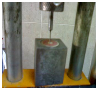
Figure (2): Sample fixed on digital universal testing machine for PBS/D.
