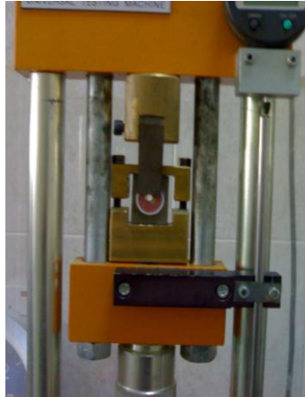
Figure (3): Sample fixed on digital universal testing machine for SBS/D.
