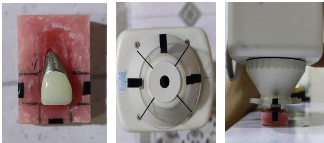
**Figure (4):** Aligning the positioning guide with the device while taking measurements
