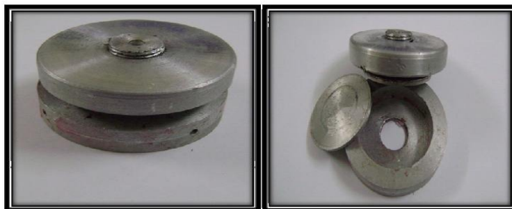
Figure (1) Aluminum mould for acrylic base resin
