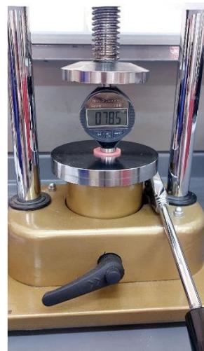
**Figure (5):** Sample under the test of Shore D hardness.
