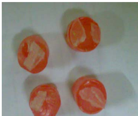
Figure(4): samples with mixed failures
