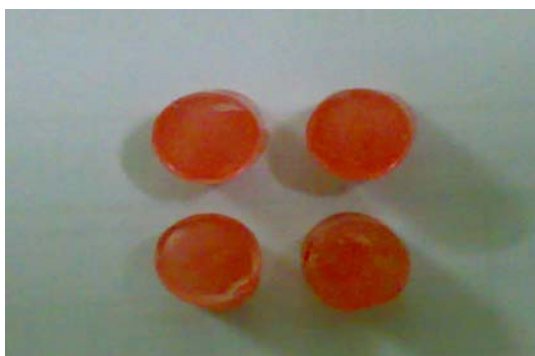
Figure (3): Samples with adhesive failures
