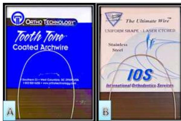
**Figure (1):** Arch wires for experimental study A: Tooth tone epoxy-coated stainless steel (Orthotechnology, West Columbia, USA). B: Fantasia non-coated stainless steel (International Orthodontic Service IOS™, Houston, USA).
