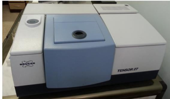
Figure (3) Fourier transform infrared spectroscopy (FTIR) (Bruker27,TENSOR, Germany)
