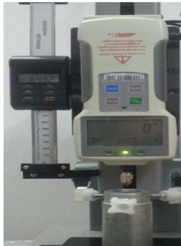
Figure (2): Digital Force Gauge Machine ( Model ZP, Imada Co., LTD. Japan)
