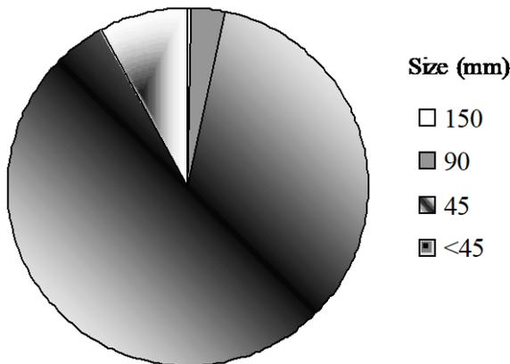
Figure (1): Weight percentage of particle size of Quayle-Dental heat-curing acrylic
