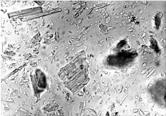
Figure (1): Microscopical examination of AL-AHLEIA plaster (Particles are irregular, fibrous and porous)
