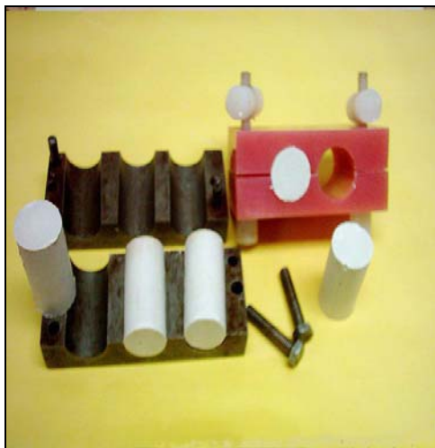
Figure (2): Split moulds with cylindrical sample
