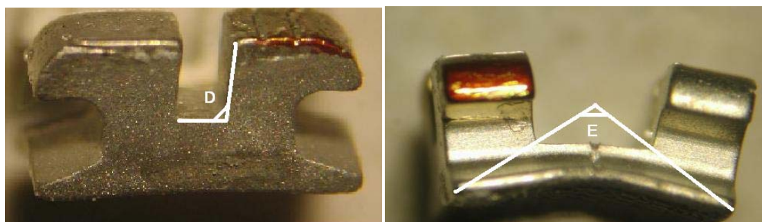
Figure (2): The stainless steel bracket dimension: (D) labio-lingual angle, (E) bracket base curvature angle.
