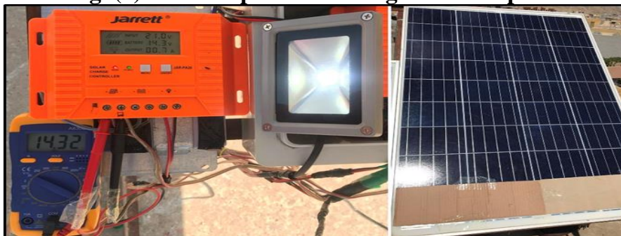
Fig. (4) The tools used to measure the effect of partial shading on the efficiency of the PV panel
