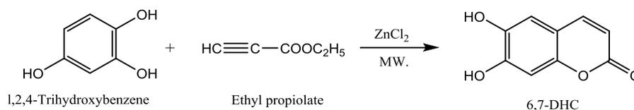
**Scheme 3.** Microwave-assisted synthesis of 6,7-DHC
