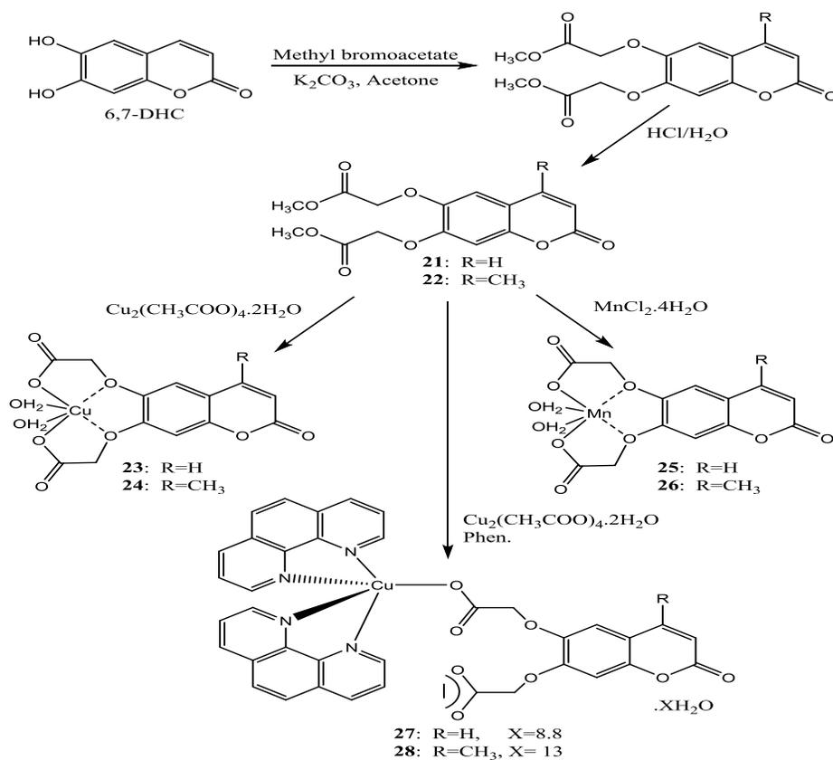
**Scheme 10.** Synthesis of coumarin-based Cu<sup>++</sup>, and Mn<sup>++</sup> salts
