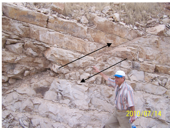
Photo 3-Antithetic reverse slip fault disrupting beds of Kometan Fm. at station 7.
