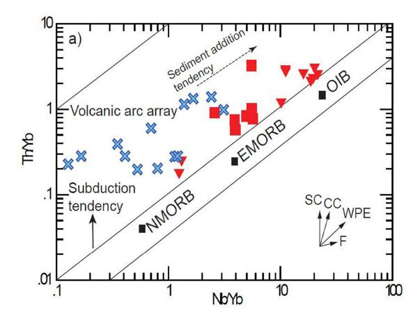
Fig. 4: Th/Yb versus Nb/Yb Diagram Indicates an Island arc Character for all Samples, Although Walash Samples Actually Belong to a Back-Arc Basin (Data from Ali *et al.*, 2012). Symbols: Filled Red Square = Walash Calc-Alkaline Samples; Filled Light Red Triangle = Walash Alkaline Samples; Blue Cross = Naopurdan Arc Samples. The Trends for WPE = Within-Plate Enrichment; SC = Subduction Zone Flux; CC = Crustal Contamination; F = Fractional Crystallization.
