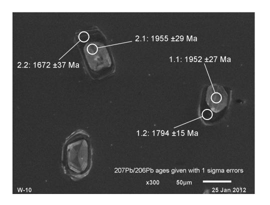
Fig. 2: Cathodoluminescence Image of Dated Zircon (GA8-GA9) Showing Location of 233 SHRIMP RG Ion Microprobe Spots with <sup>207</sup>Pb/<sup>206</sup>Pb Ages. Circles Indicate spot Location; Ages Indicated in Ma, Illustrating the Presence of Both Light and Dark CL Core and Rim Domains (i.e. Low and High U, Respectively).
