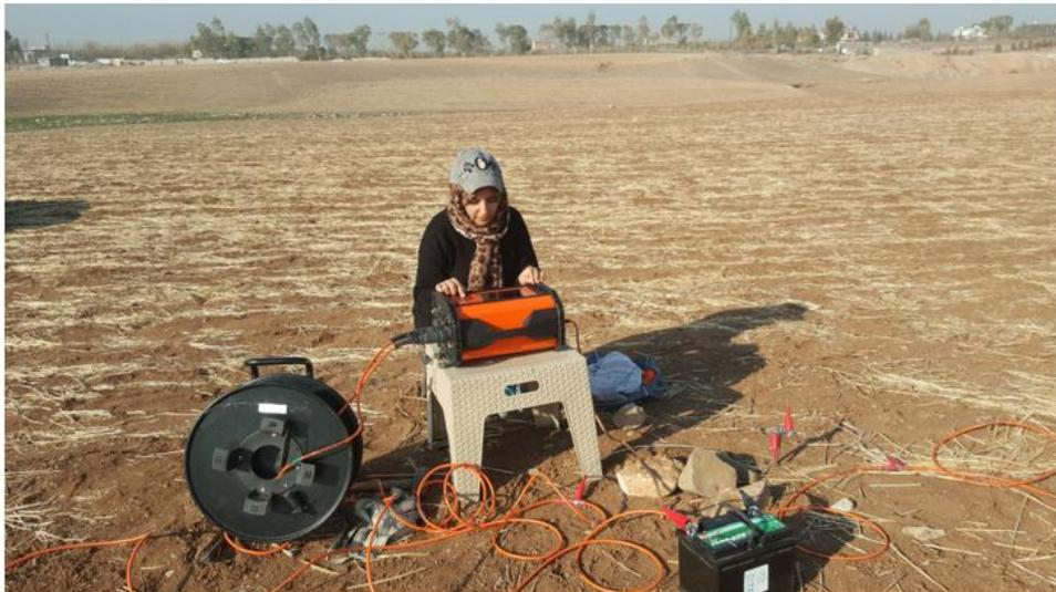
**Fig.4. Fieldwork imaging survey with Terrameter LS system**
