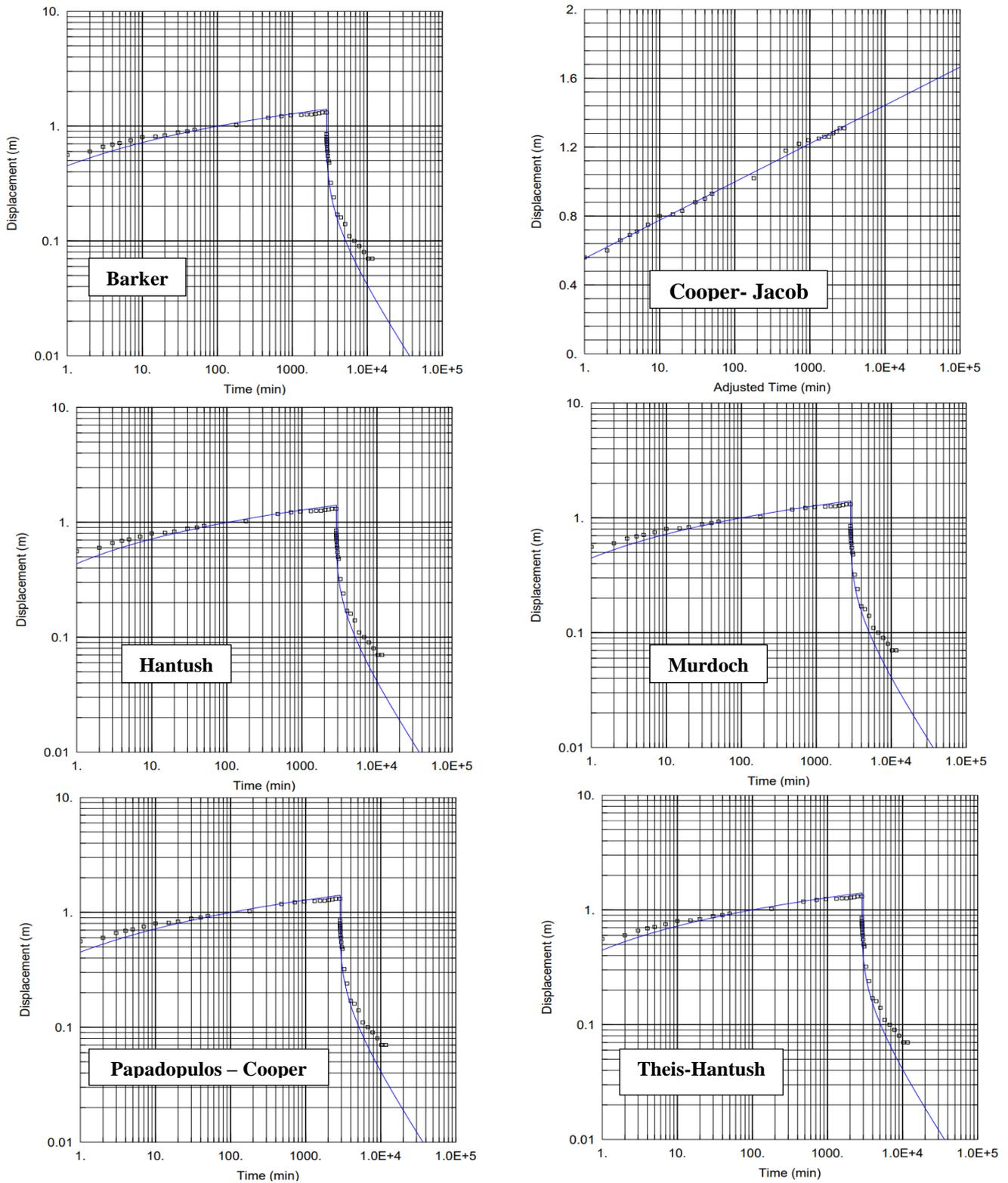
Fig. 3. The results of the pumping test graphic presentation for the methods used
