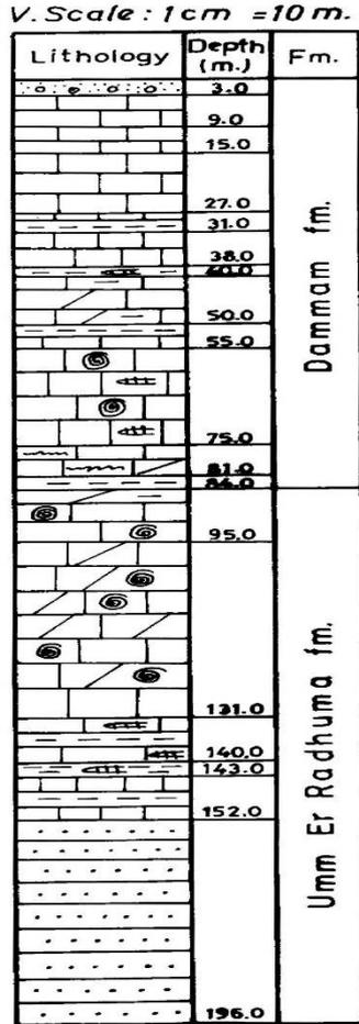
Fig. 2. Vertical section for the well (B7-3), after (Consortium, 1977)
