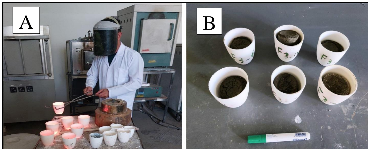
Fig. 4. A-Samples after burning, B-Clinker product.
