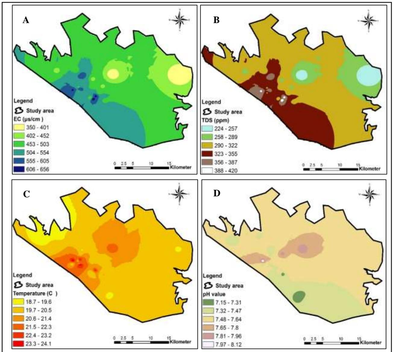
Fig. 5. Distribution map of physical parameters in the second period; A-Electrical Conductivity, B- Total Dissolved Solid, C- Temperature, and D- pH value.
