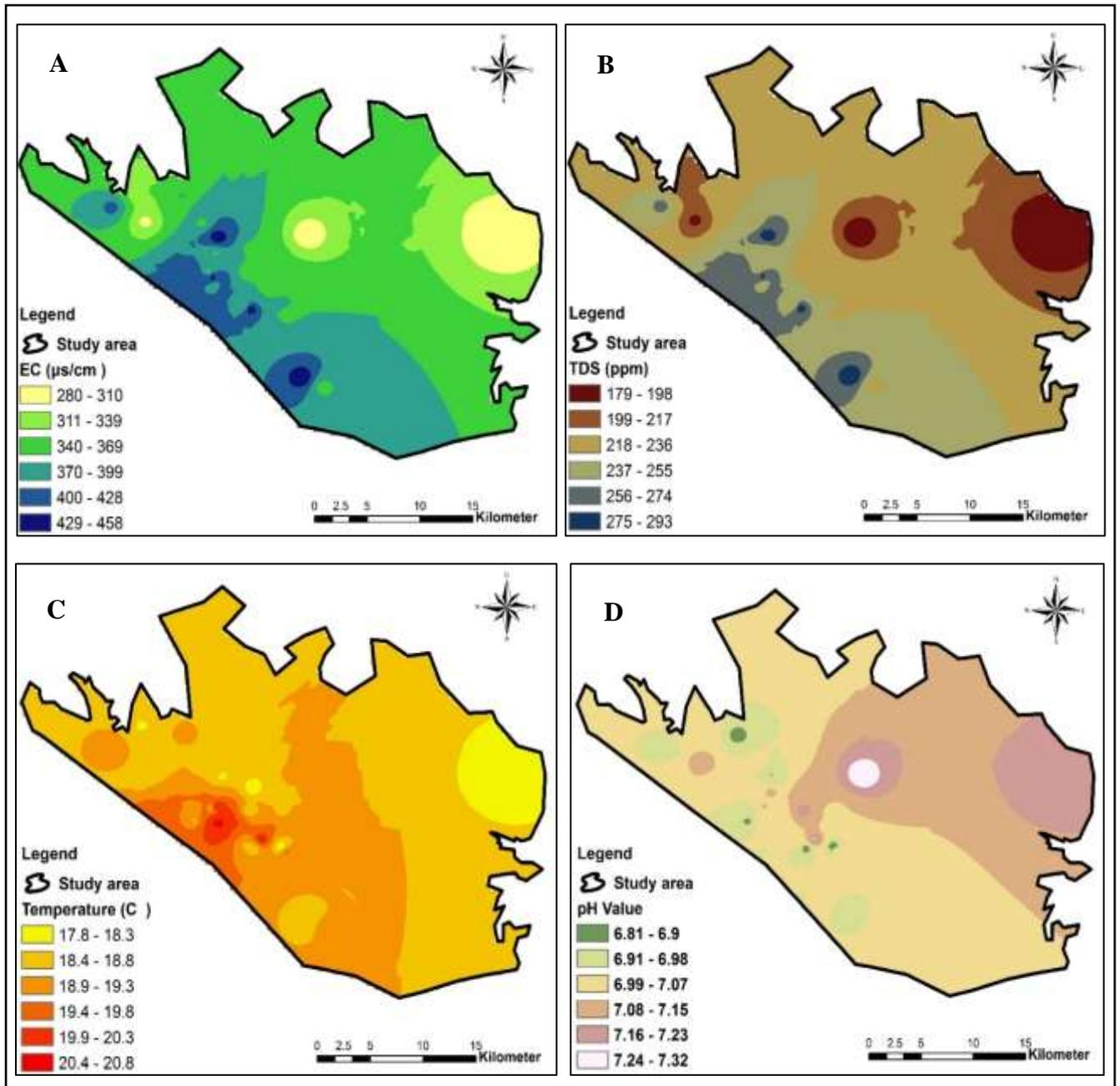
Fig. 4. Distribution Map of Physical Parameters is First Period; A-Electrical Conductivity, B- Total Dissolved Solid, C- Temperature, and D- pH Value.
