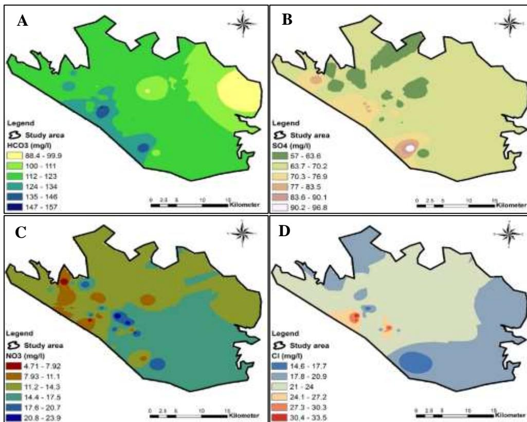
Fig. 8. Distribution map of anions concentration in the first period; A- Bicarbonate, B- Sulphate, C- Nitrate, and D- Chloride.
