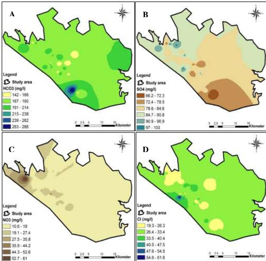
Fig. 9. Distribution map of anions concentration in the second period; A- Bicarbonate, B- Sulphate, C- Nitrate, and D- Chloride.
