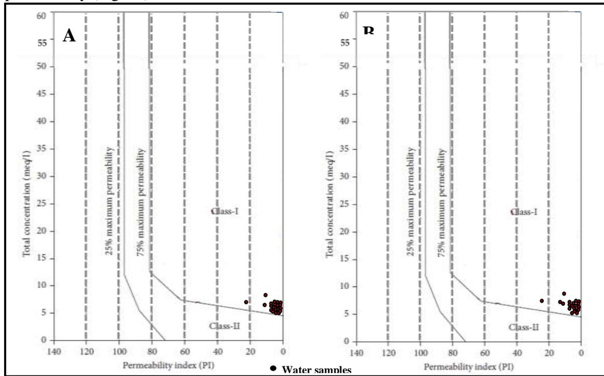
Fig. 10. Permeability index diagram classification of the groundwater quality.
