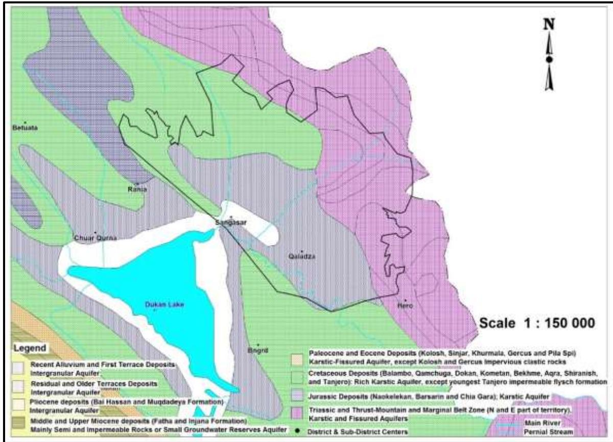
Fig. 2. Aquifer system and type of deposits in the study area (After Stevanovic, 2003).
