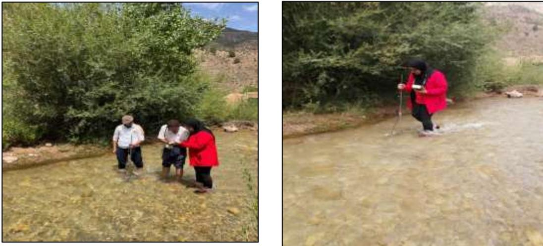
**Photo panel. 1. Measurement of River flow using the micro-current meter**
