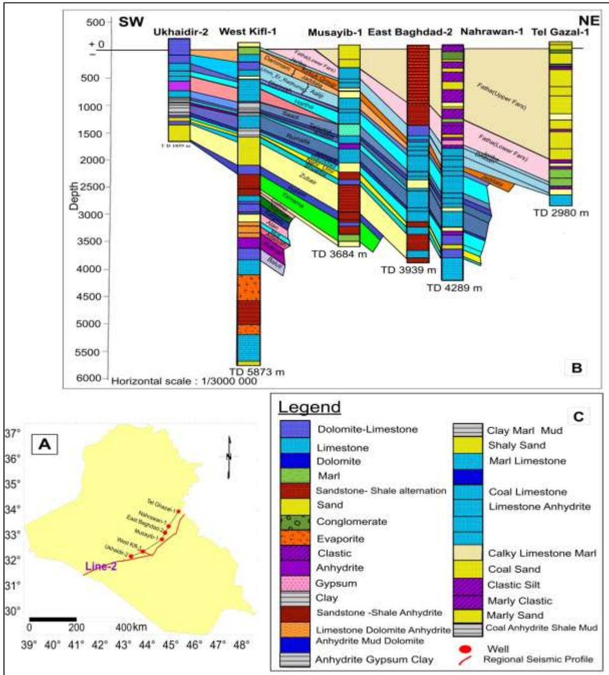
**Figure 3. (A) Location of the considered wells, (B) The correlations between the formations along the study area, (C) Legend showing the lithology of subsurface formations (modified After O.E.C., 1989).**
