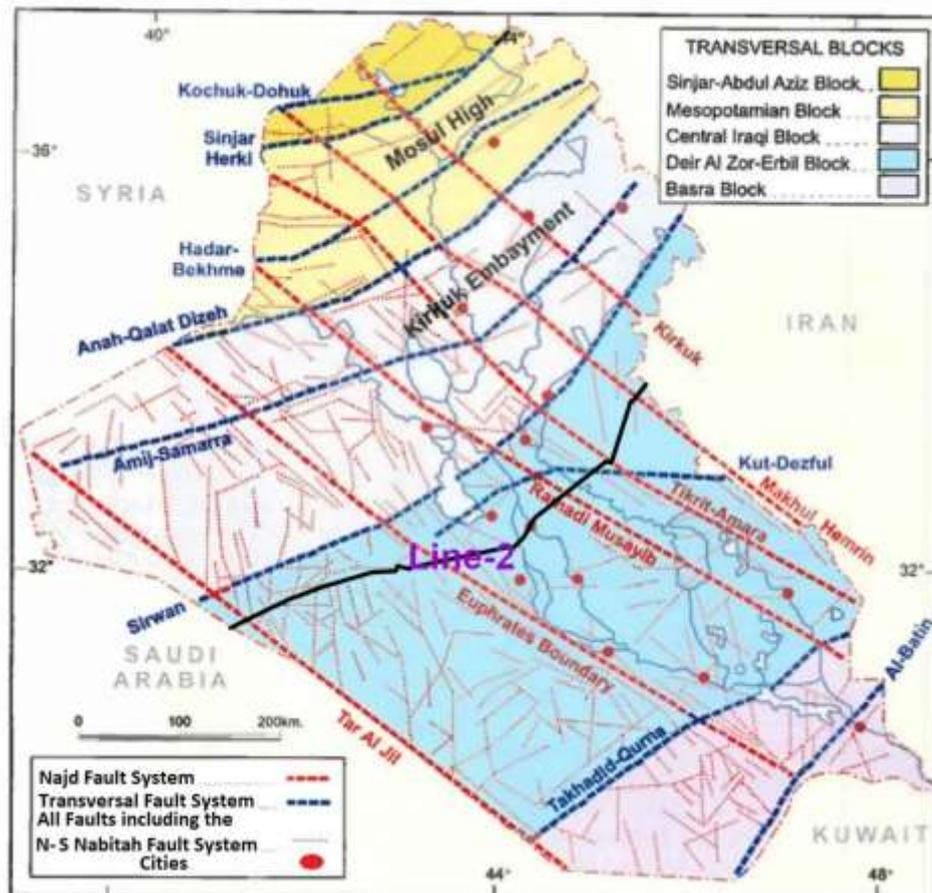
Fig. 4. The regional seismic section crossing many regional NW-SE faults traced on the tectonic map of Iraq prepared by Jassim and Goff, (2006).
