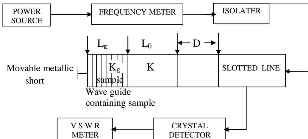
Fig. 1-A : Two Point Method of Measuring Dielectric Constant at  $\lambda = 2.8\text{cm}$ .
