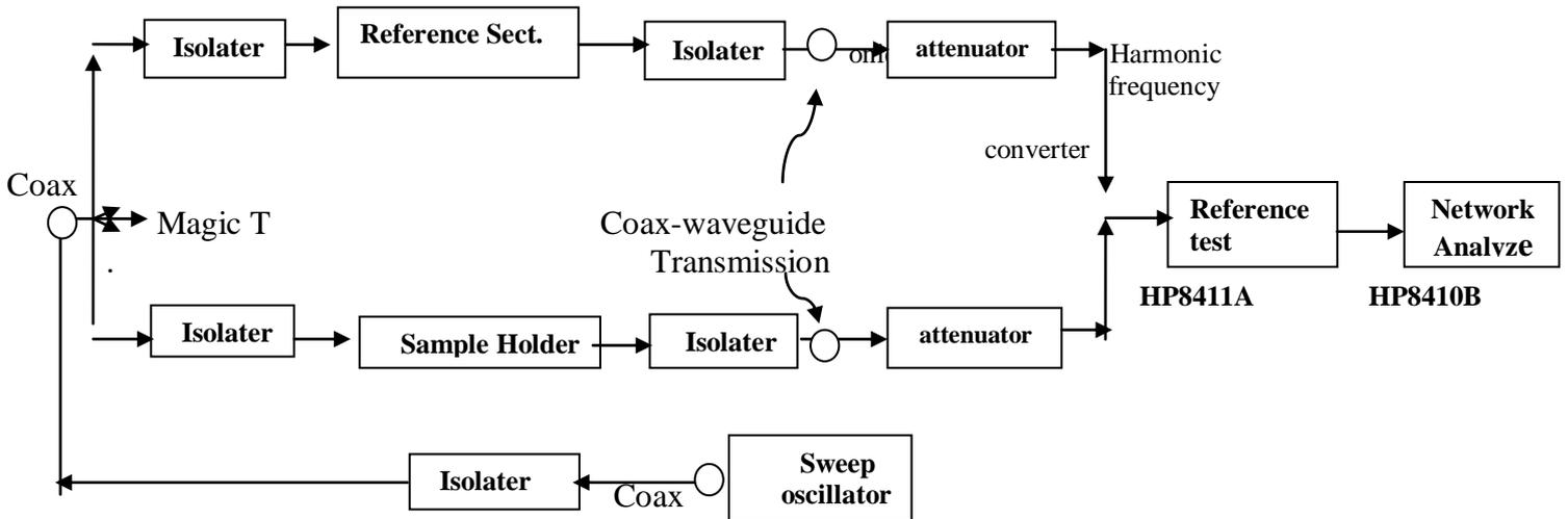
Fig. 1-B: Block Diagram of the Dielectric Measurement System at  $\lambda = 21\text{cm}$ .
