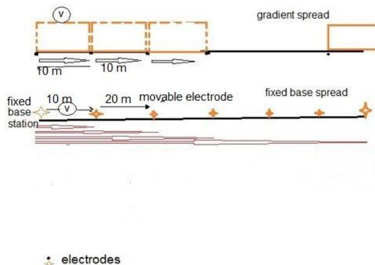
Fig.2. The SP electrodes layout schemes
