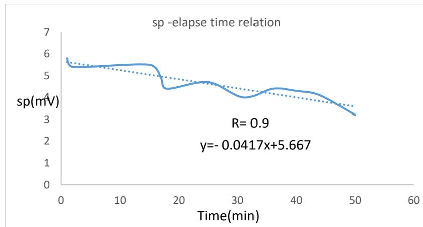
**Fig. 10. Correlation between the elapse time with SP measurements in the pumping test**
