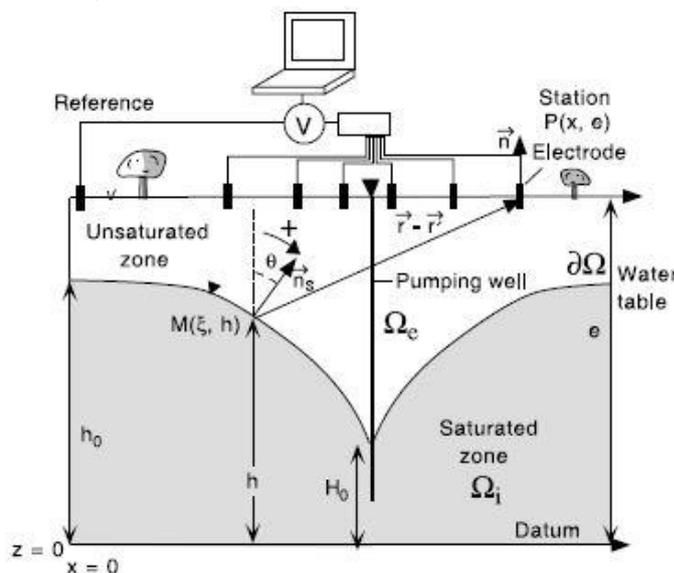
Fig. 9. Pumping test procedure and SP monitoring Scheme (after Rizzo et al ,2004)
