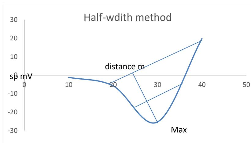
**Fig. 12. Half-Max Depth interpretation method for SP gradient line2**
