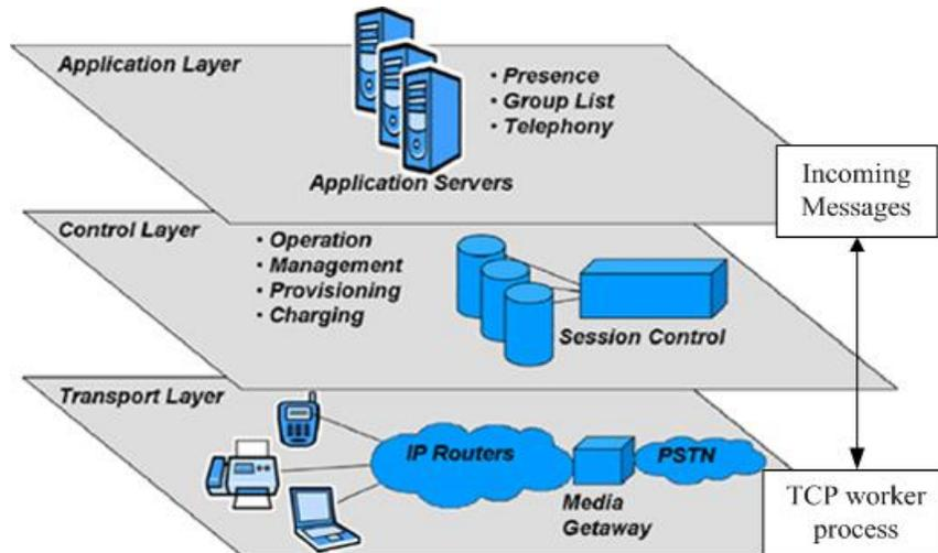
**Figure 1.** IMS architecture layers
