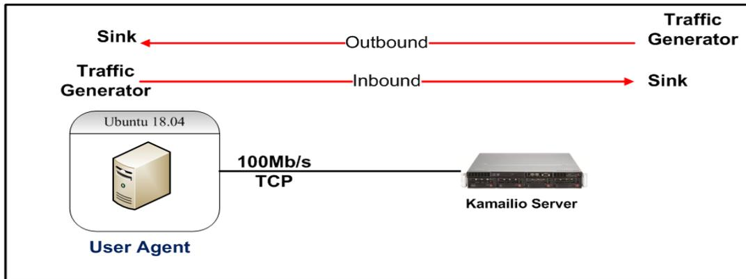
**Figure 4.** Network topology for the experiment
