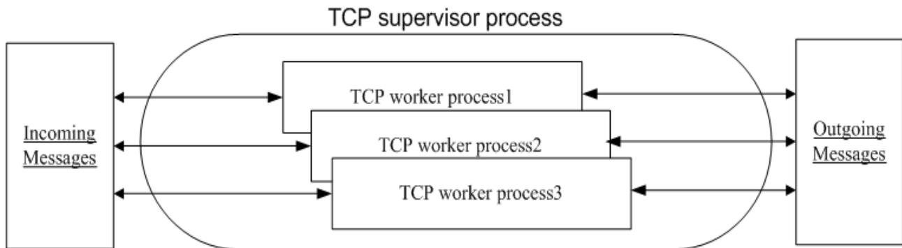
**Figure 3.** TCP workers process and supervisor
