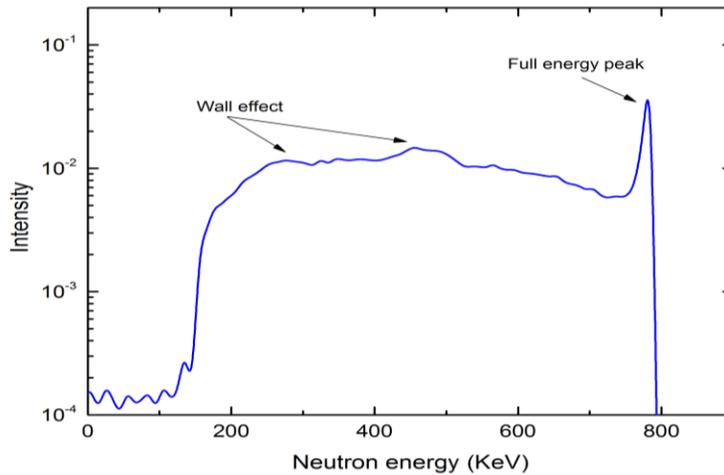
Figure 5. Pulse height spectrum of the  $^3\text{He}$  detector
