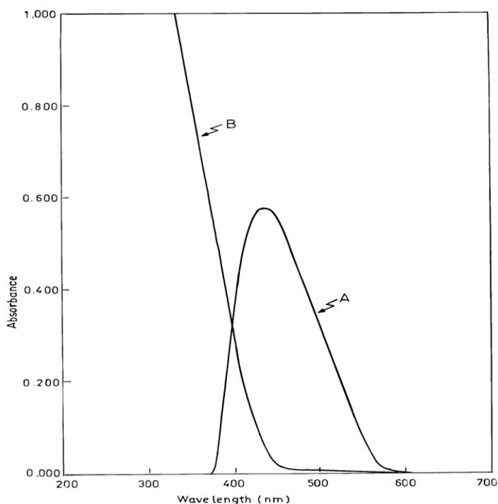
**Fig 3. Absorption spectra of 3 µ g ml<sup>-1</sup> of tranexamic acid measured against reagent blank (A) and the reagent blank measured against distilled water (B) with diazotised sulphanilic acid**
