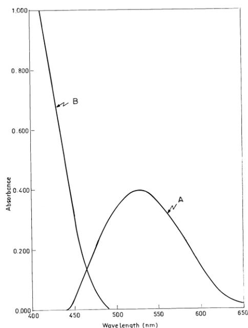
**Fig. 4.** Absorption spectra of  $3 \mu\text{g ml}^{-1}$  of tranexamic acid measured against reagent blank (A) and the reagent blank measured against distilled water (B) with diazotised p-nitroaniline
