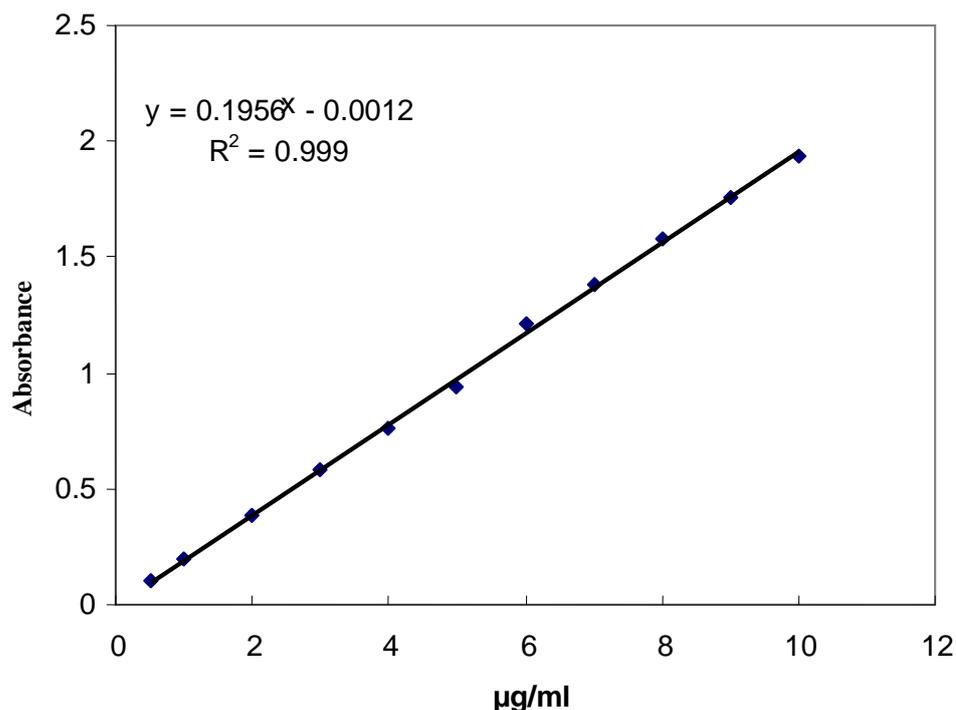
**Fig. 1. Calibration graph for the determination of tranexamic acid with diazotised sulphanilic acid**
