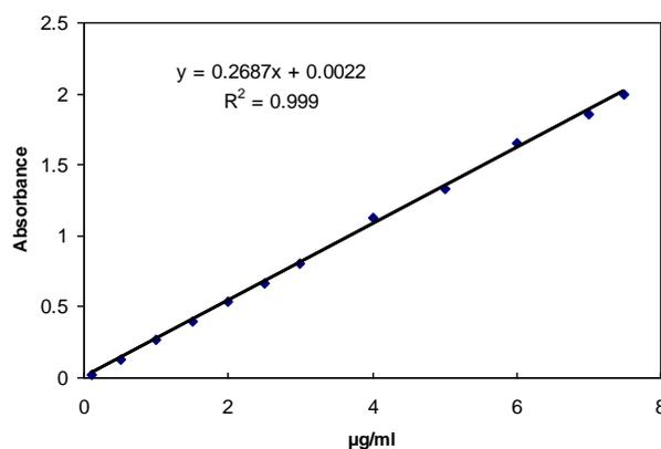
**Fig. 2. Calibration graph for the determination of tranexamic acid with diazotised p-nitroaniline**
