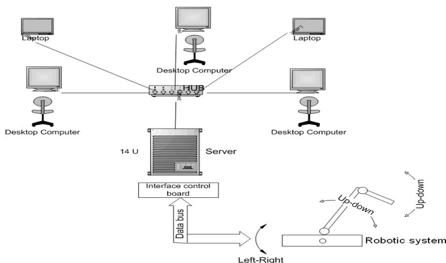
**Fig. (1) Robotic system remotely connected through LAN.**
