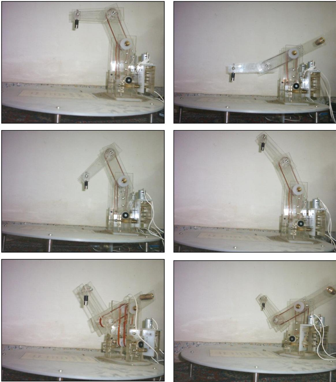
**Fig. (6) Three-joint Robotic system in different movements.**
