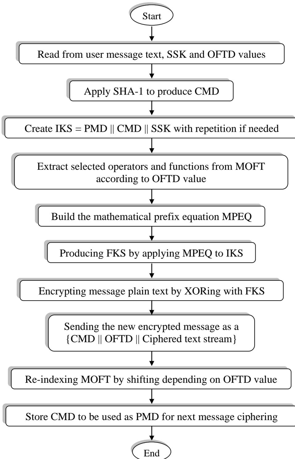
Figure. 5. Flow chart of proposed sending algorithm
