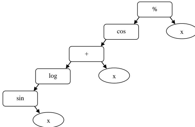
Figure. 3. Prefix mathematical equation with inserted arguments
