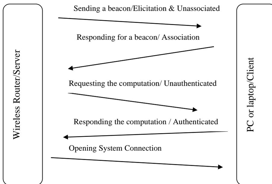
Figure 3: Traffic Protocol Authentication Module
