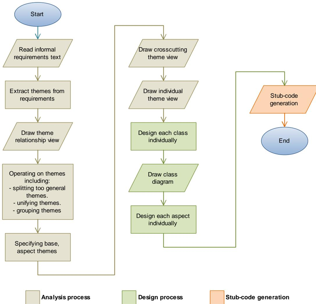
Figure 3: RADC-AO tool flowchart.
