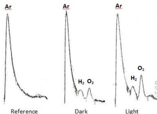
**Figure 2.** GC traces gas for the optimized performance of PEDOT/nano-Ni confirm O<sub>2</sub> gas was the main gas that evolved
