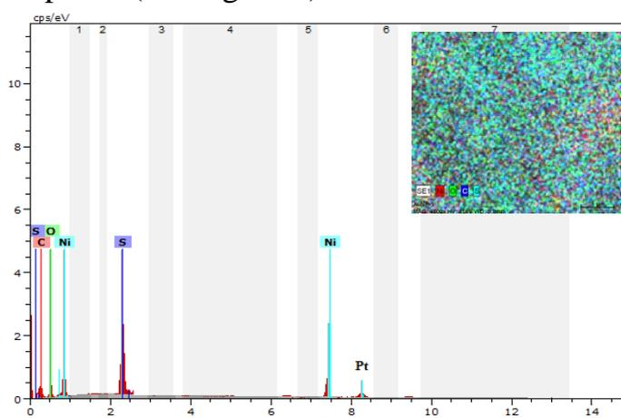
**Figure 3.** EDX spectrum of PEDOT/nano-Ni confirms the composition, the inset picture shows the uniform mapping distribution.
