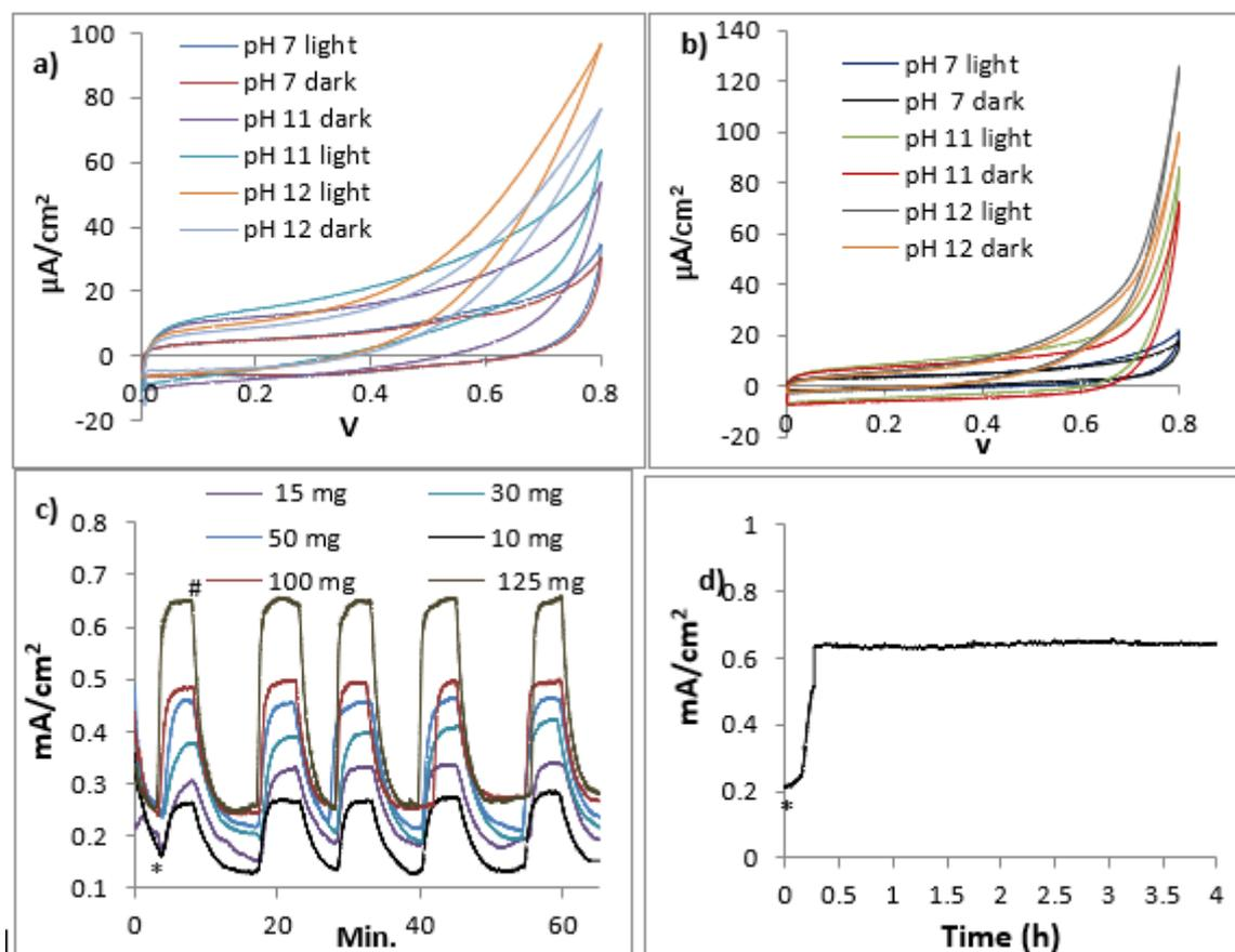
Figure 1. (a) CV of PEDOT under varying pH conditions. (b) CV of PEDOT/nano-Ni films with minimum concentration of nano-Ni (5 mg) with similar condition that applied in Fig.1(a). (c) Chronoamperograms of PEDOT/nano-Ni (with different nano-Ni concentration in polymerization solution) over 1 h of operation with and without light illumination of 0.25 sun (\* = 'light on', # = 'light off'). (d) Chronoamperogram over 6 h of operation.
