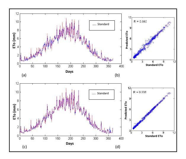
Figure (4). Time series plots (a and c) and scatter plots (b and d) of validation phase (case 10) for the standard and predicted ETo values in mm/day, (a and b) without time index, (c and d) with time index.
