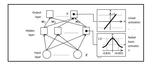
Figure (3): A schematic diagram of RBF network
