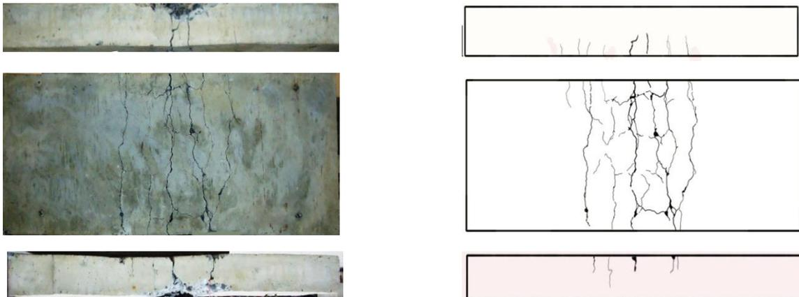
Fig 14: Cracks Pattern of Control Slab (A)
