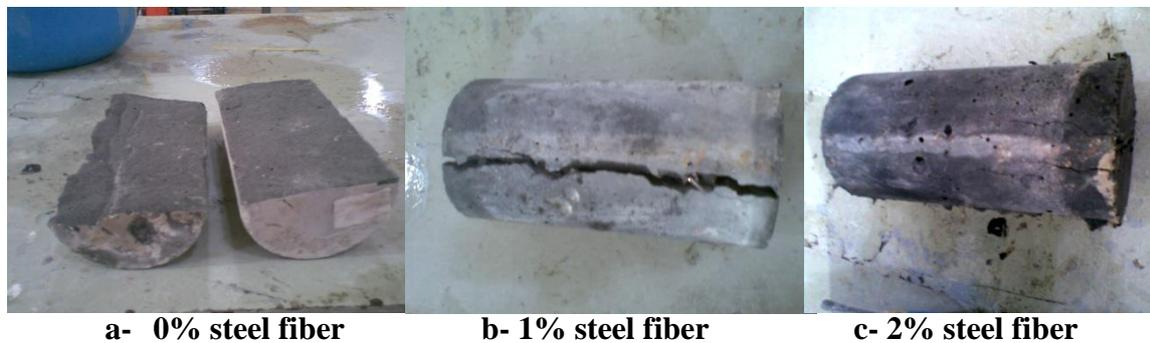
**Fig.(3)The specimen after splitting test**
