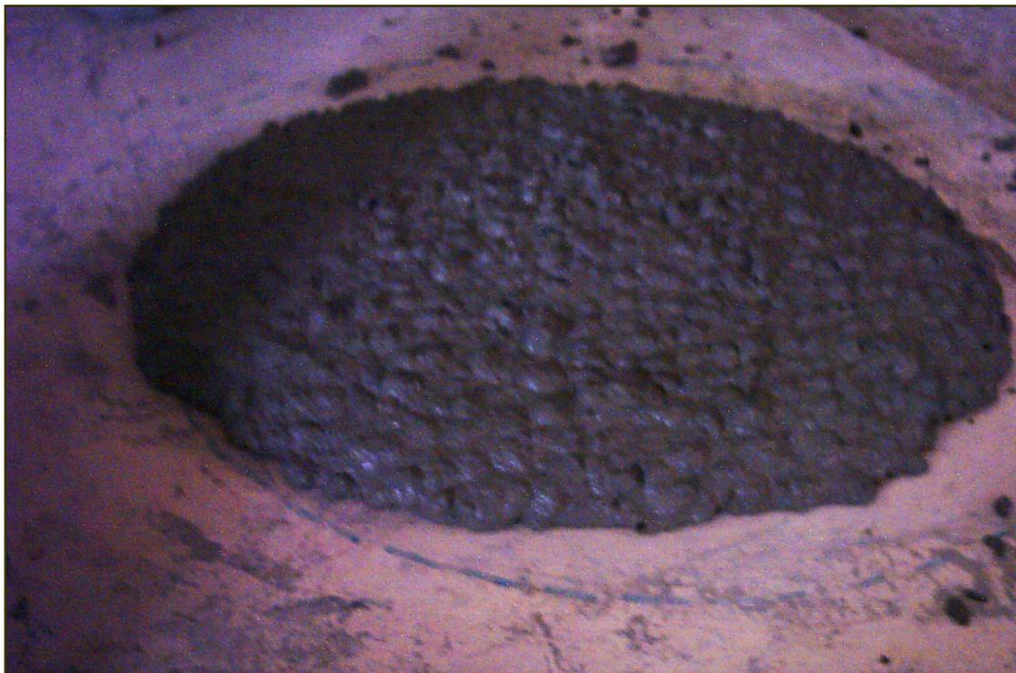
**Fig. (1) Flow Test of SCC concrete.**
