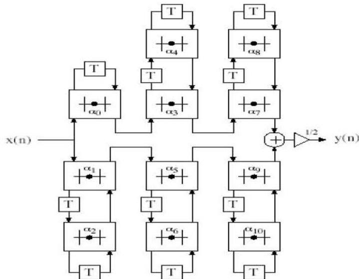
Fig. 2 An 11<sup>th</sup> order lattice wave digital filter.
