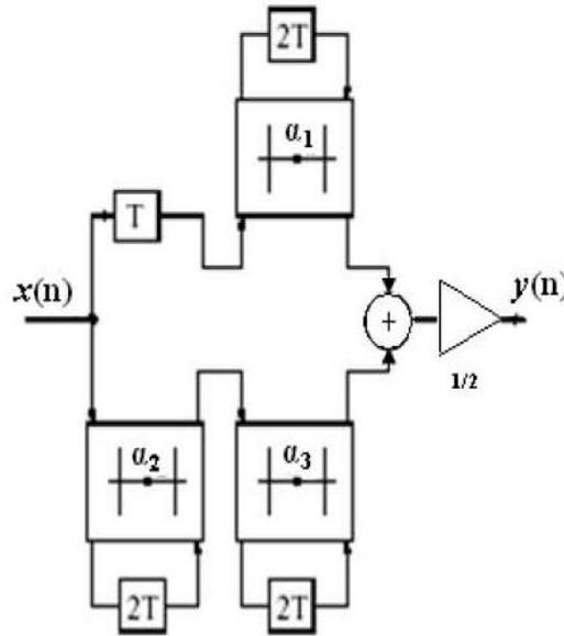
Fig. 3 A 7th-order bireciprocal lattice wave digital filter.
