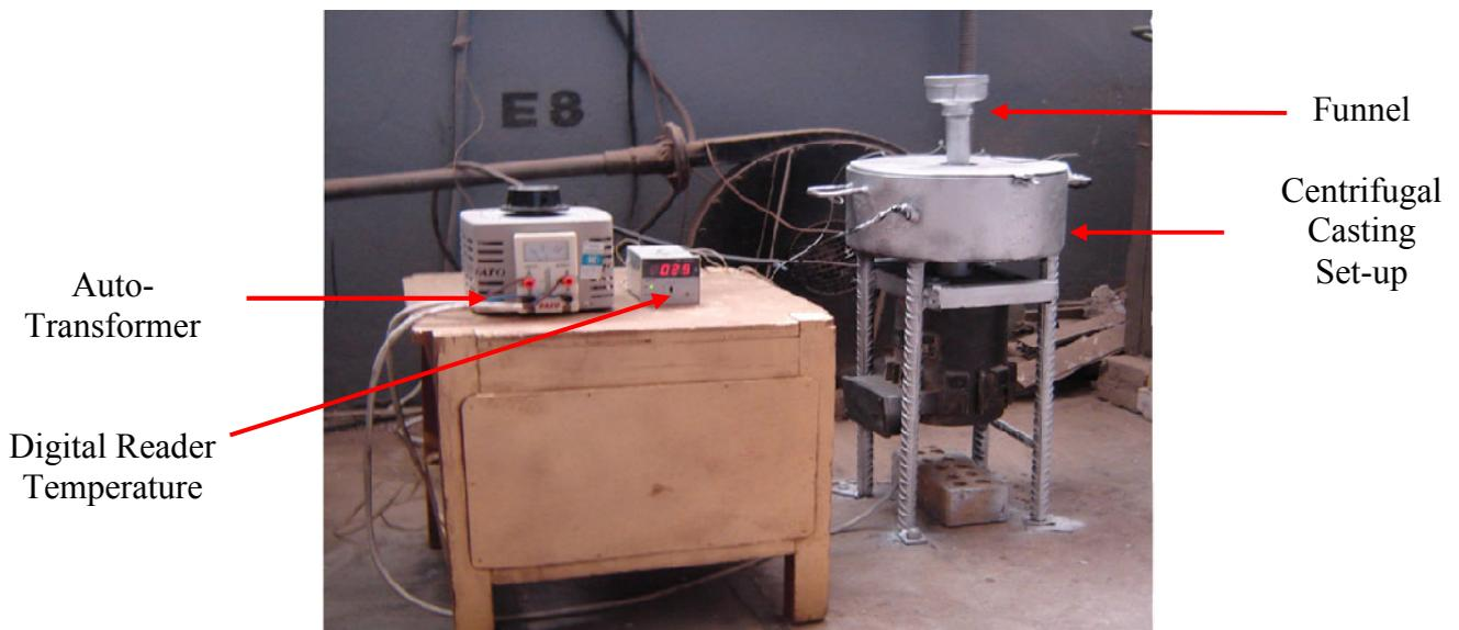
**Figure (2):** Photograph of centrifugal casting apparatus.
