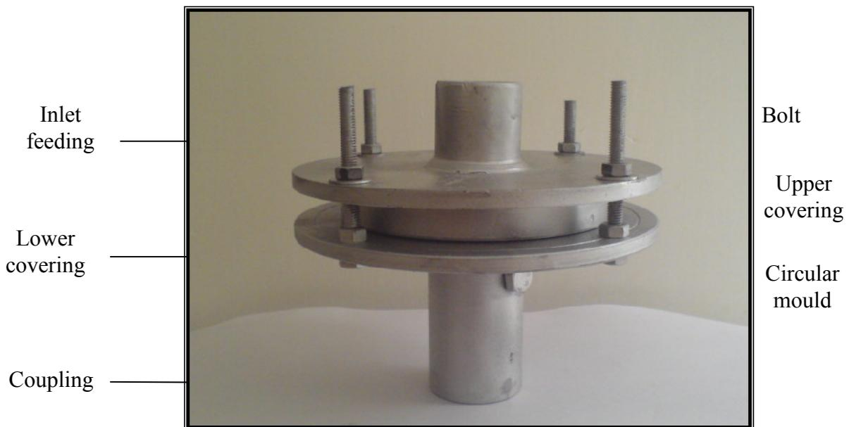
**Figure (4):** Photograph of the assembly of mould.
