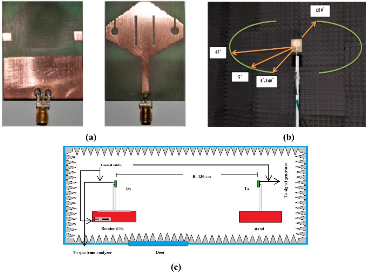
(a). Printed antenna (b). Antenna in an anechoic chamber
