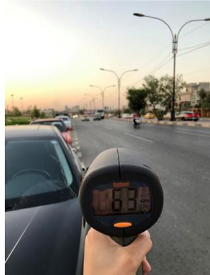
Fig. 4 Radar speed gun.
