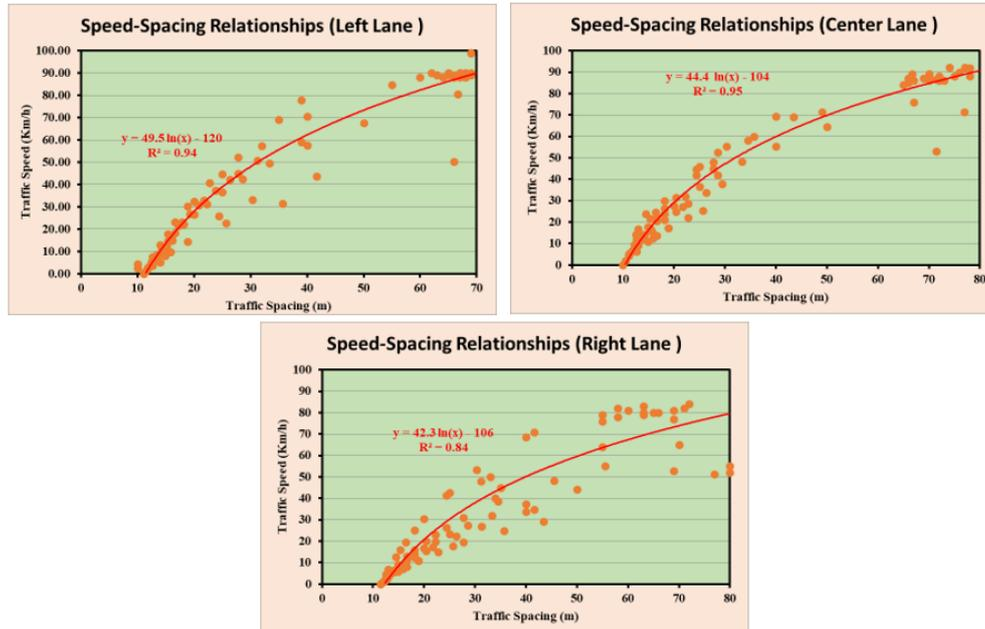
Fig. 6 Logarithm relationship and mesoscopic model between space mean speed and traffic spacing for each lane of segment NO.1, North dir. with R-square values.
