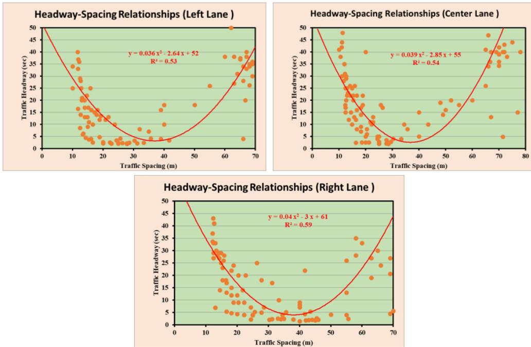
Fig. 8 Quadratic relationship and microscopic model between time headway and spacing for each lane of segment NO.1, North dir. with R-square values.
