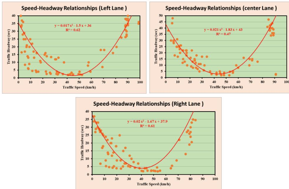
Fig. 7 Quadratic relationship and mesoscopic model between space mean speed and time headway for each lane of segment NO.1, North dir. with R-square values
