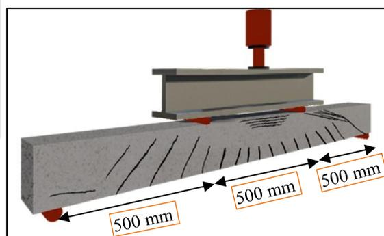
Figure 9: 3D drawing for the four-point flexural test.
