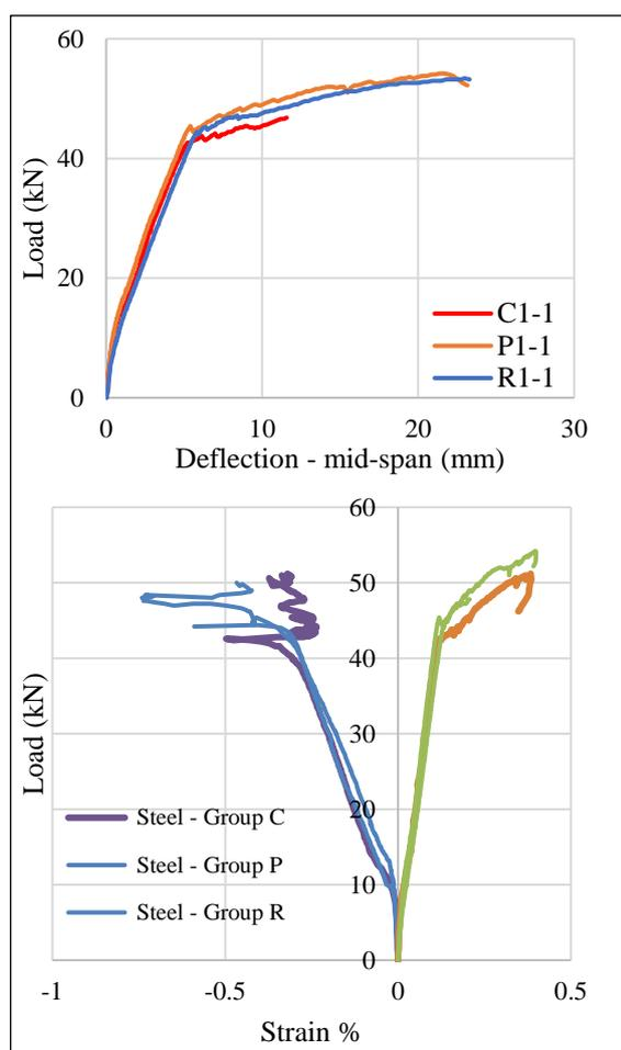
Figure 11: Load-deflection for RC samples without CFRP strengthening.
