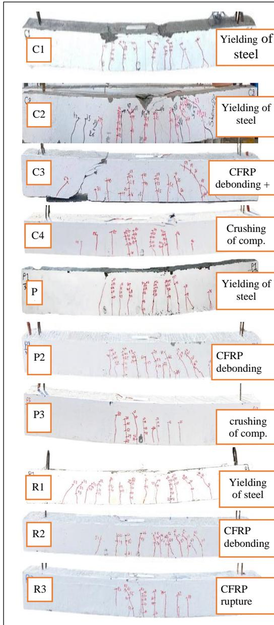
Figure 15: Failure mode
