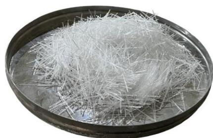
Figure 2: Polypropylene plastic fiber.
