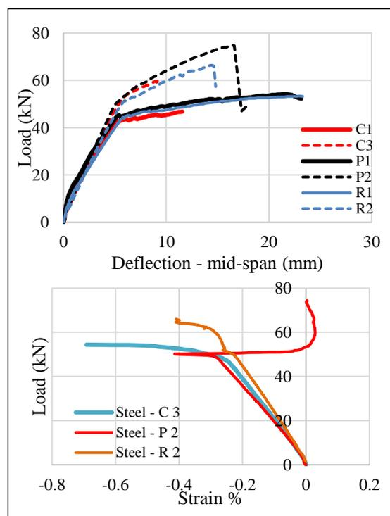
Figure 12: Load-deflection for RC samples with fiber addition.
