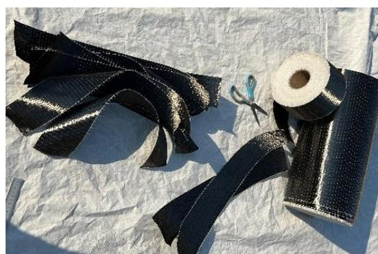
Figure 3: CFRP composite.
