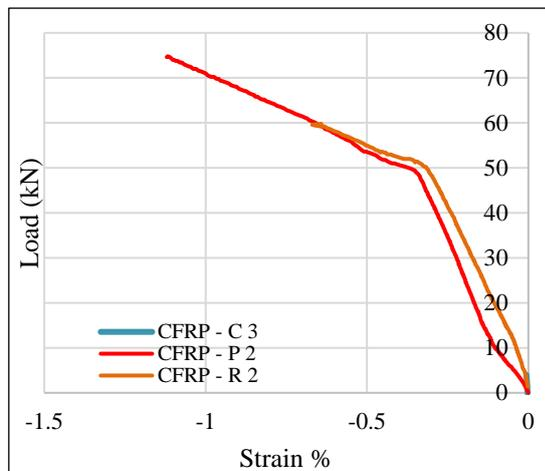
Figure 13: Strain level in steel and CFRP for C3, P2, and R2.
