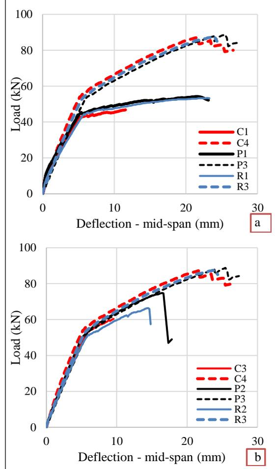
Figure 14: Load-deflection for RC beams with end-anchorage vs non anchorage
