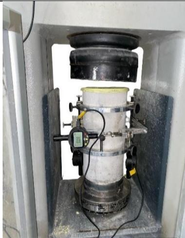
Figure 10: Cylindrical sample under compression machine test.
