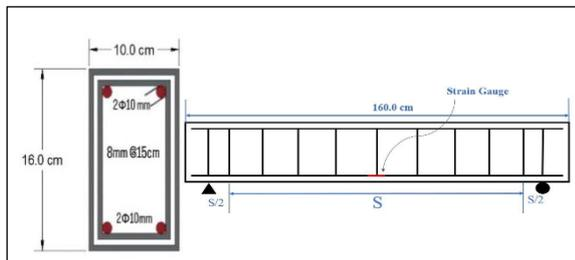
Figure 4: Section reinforcement detailing.
