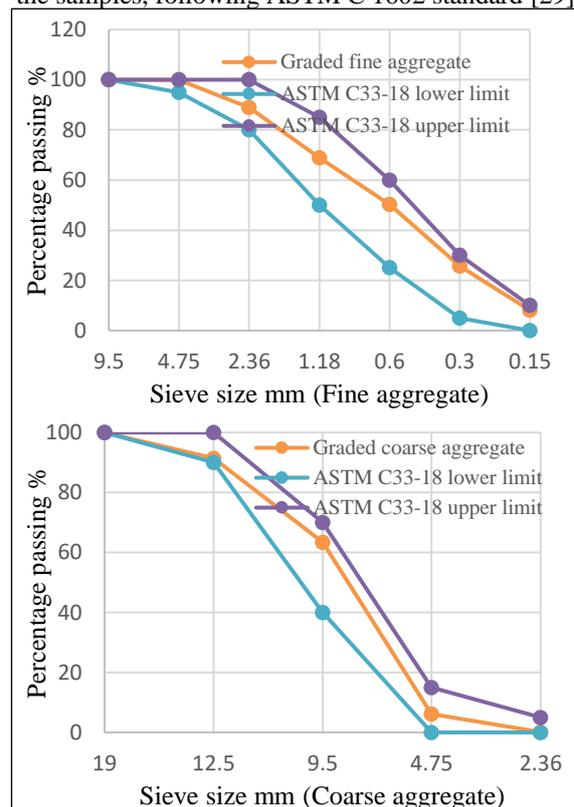
Figure 1: Aggregate sieve analysis.
