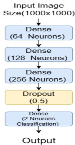
Fig. 4 The architecture of the proposed FNN scheme.
